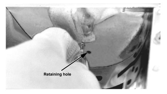
Figure 21. Removing or Replacing the Bulb
